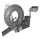
3. According to the size of the tire which needs to be repaired, to adjust the spreading claw to be the appropriate height. Place the spreading hook to link pin of the hanging device. Adjust the spreading hook up and down in order to insert into one of the adjusting holes which have 7 groups total. Put the short spread hook inside the tire and try to place the tire in the middle of tire lever if possible.
