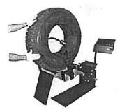
7. The work light fixed on the machine needs to be adjusted to a proper position, to illuminate the inside sufficiently and make the repair work easy.
