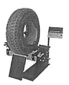
8. After finished maintenance work, please firstly move the up & down control valve to the downward direction, let the tire fall to the lowest, then move the up & down control valve to the direction of contraction, loosen the spreading hook and remove it from the tire core, then discharge the tire along the sloping board.
