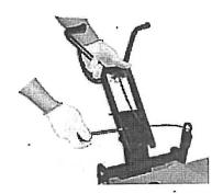
4. Pull the spreading control valve to the direction of spreading, and spread the tire to the width needed. The tire will probably disengage from the spreader if the spreading hook arm is too high. Operate after it is lowered and the height is properly adjusted.
